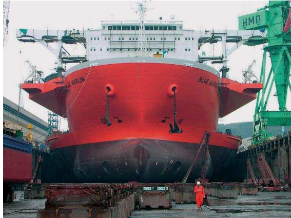
Figure 7. Hull widening of heavy transport vessel Blue Marlin (courtesy Dockwise).
